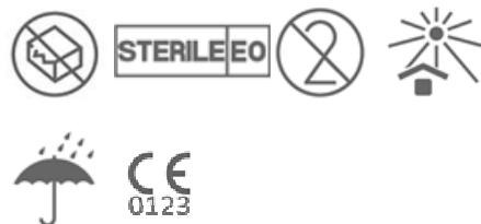
Marking on all packaging levels with CE and according to DIN EN ISO 15223-1- and DIN EN ISO 20417
